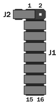
MON08 Connector Jumpered for Standalone Mode Operation
