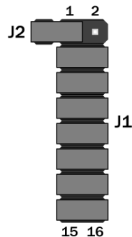
MON08 Connector Jumpered for Standalone Mode Operation
